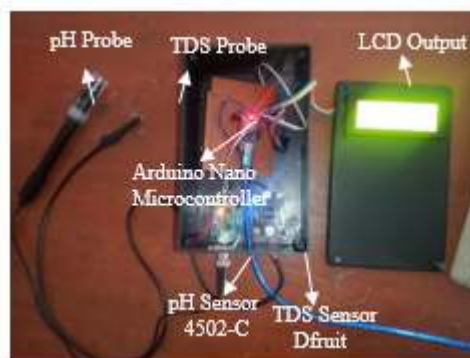
Figure 3. Water Quality Test Equipment
