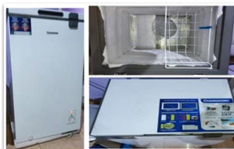
Gambar 1. Mesin chiller suhu ( -10^{\circ}\text{C} )
